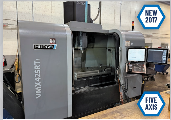
Hurco Model VMX42SRTi CNC Five-Axis VMC w/ Built in Rotary Table, High Pressure Coolant Through Spindle
