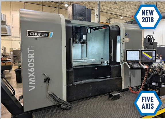
Hurco Model VMX60SRTi CNC Five-Axis VMC w/ Built in Rotary Table, High Pressure Coolant Through Spindle
