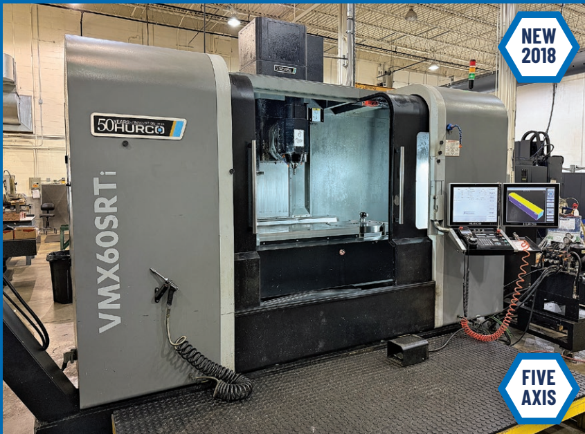
Hurco Model VMX60SRTi CNC Five-Axis VMC w/ Built in Rotary Table, High Pressure Coolant Through Spindle
