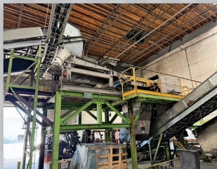
Bottle Section Sorema Eddy Current Sorting System
