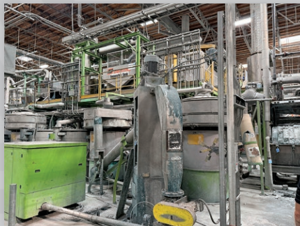
Sorema High-Capacity High-Intensity Wash Line
