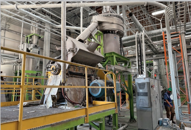
125-KW Sorema Previero Model MU-515PR Dry Grinder w/ Screener
