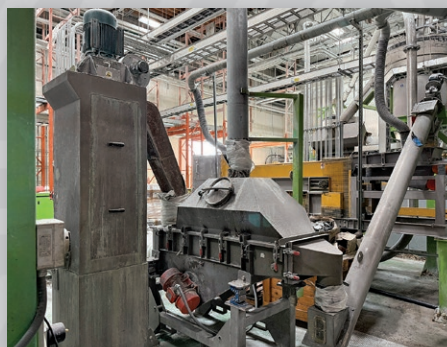
Green Flake Wash Section, Dry Section and Eddy Current Separating System
