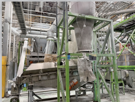
Sorema 128" x 32" Fluid Bed Dryer on clear line
