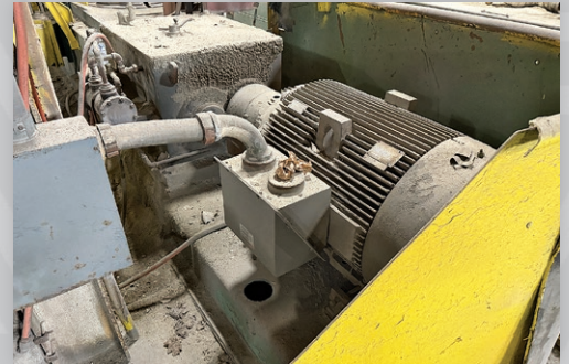
Morgan 2-Block Wire Drawer, 24" Blocks / 30" Finishing Block, 250-HP, ABB Drive
