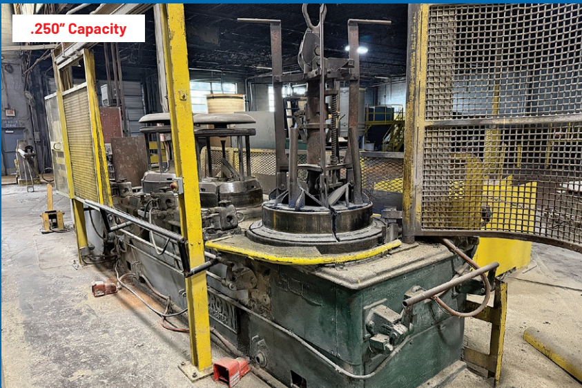
Morgan 2-Block Wire Drawer, 24" Blocks / 30" Finishing Block, 250-HP, ABB Drive
