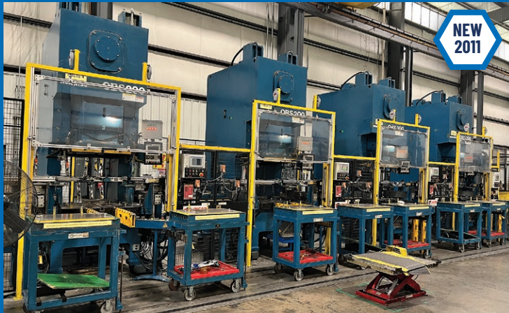
(4) 220 Ton Komatsu Model OBS200-61 Single Crank Gap Frame Press; 25-50 SPM, 11.8" Stroke
