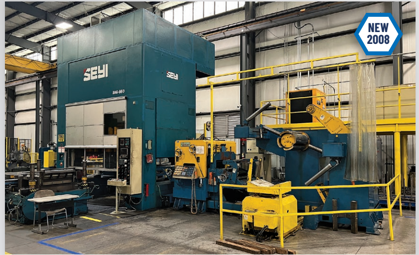
660 Ton Seyi Model SAG-660 SSDC Press; 9.84" Stroke, 30-60 SPM
