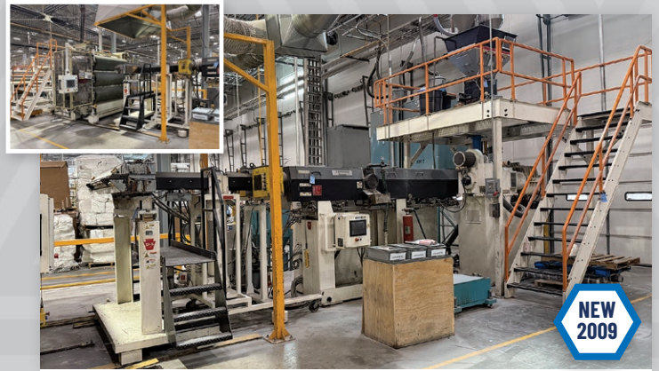
80" Davis-Standard Sheet Line, 300-HP, 76" Sheet Die, Pull Rolls, Shear
