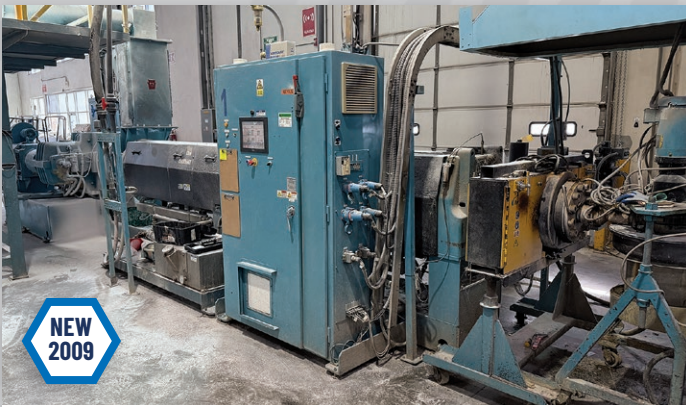
6" Davis-Standard Compounding Line w/ Pelletizer, 500-HP, Screen Changer
